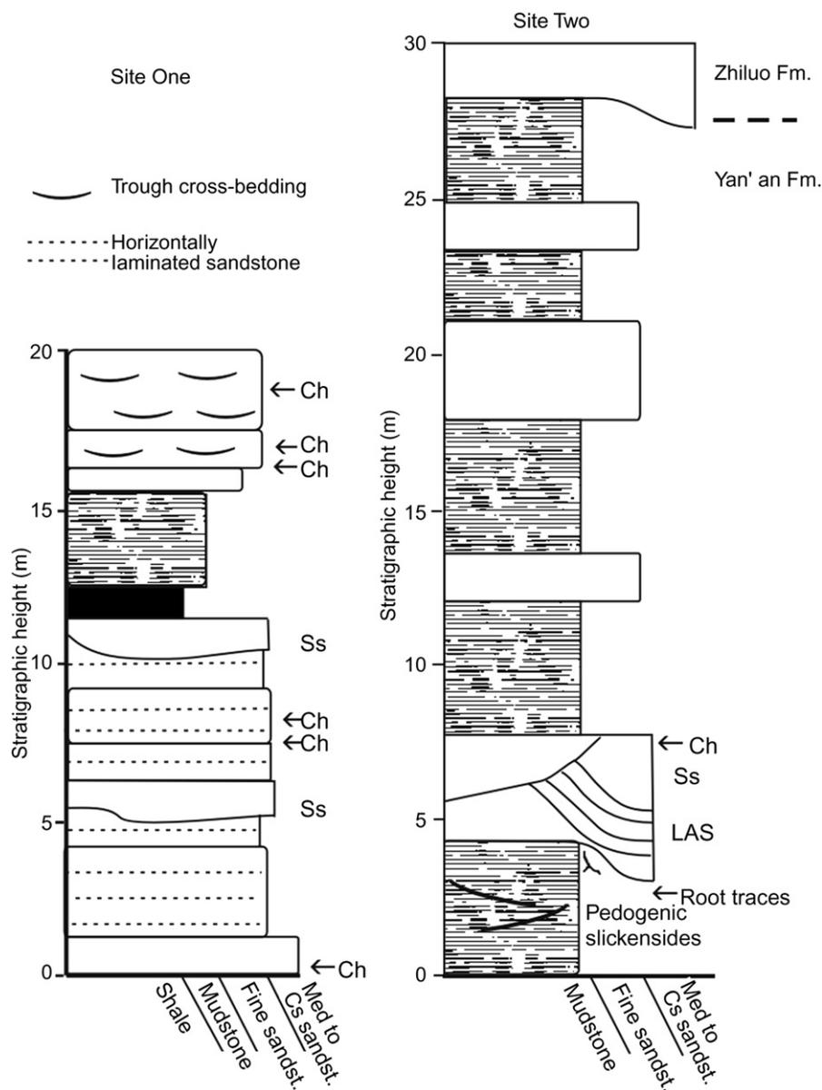
**Figure 2** Stratigraphic sections measured at Site One (Member Two) and Site Two (Member Four and its contact with the Zhiluo Formation). Occurrences of fusain (Ch) are indicated for each section. Sandstone scour surfaces (Ss) are notable in the section at Site One, and lateral accretion surfaces (LAS) occur in the outcrop at Site Two.
