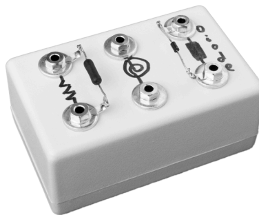
Figure 1 The banana plug circuit board holding the resistor, the light bulb, and the diode. The resistor and diode can be seen on the top of the box, while the light bulb is mounted inside. The orientation of the diode is not known in advance but must be determined from the data.
