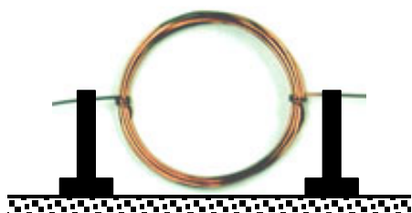
Figure 5 Make this coil as a first step in building an electric motor. The posts show how the coil will be supported as it rotates.
