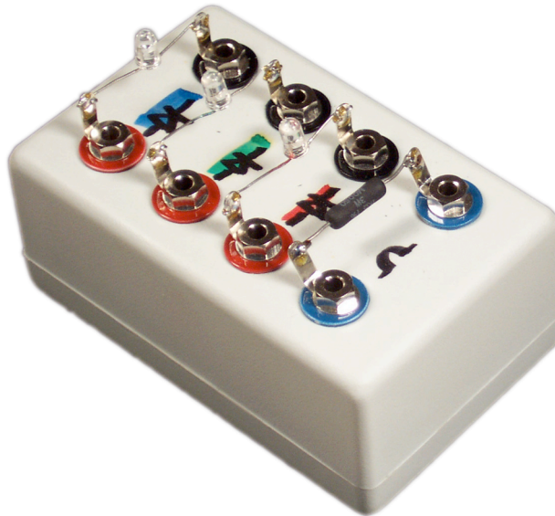
Figure 9 The banana plug test board used in these lab activities. Note the 1 k \Omega resistor and the three LEDs.
